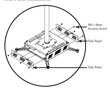
**Step 1.** Attach the two side panels using eight (8) M4 x 8mm security screws.
